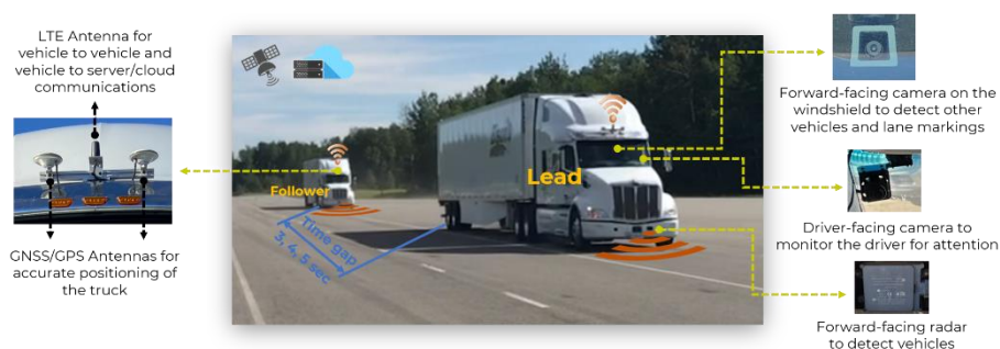
Fig. 1. Equipment and sensors used in cooperative truck platooning.
